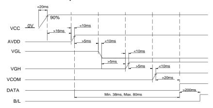
Power on sequence:  $VCC \rightarrow AVDD \rightarrow VGL \rightarrow VGH \rightarrow VCOM \rightarrow DATA \rightarrow B/L$
