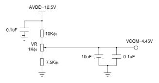
The typical VCOM is only a reference value. It must be optimized according to each TFT. Please use a VR and refer to the application circuit at left.
