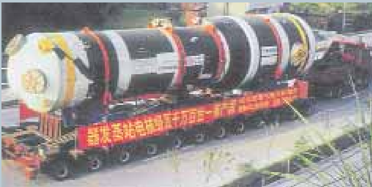
Steam generator on its way to the Chinese nuclear power plant unit Ling Ao 2
