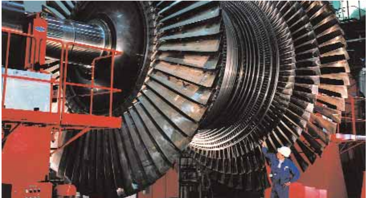
A low-pressure turbine rotor at Isar 2. At Olkiluoto 3 the last turbine stage will have a diameter of around 7 meters (m) and a blade length of 1.8 m.
